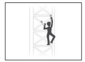
The ABSORBICA-Y lanyards with two arms allow for continuous protection, by successively detaching and re-attaching the two arms.
